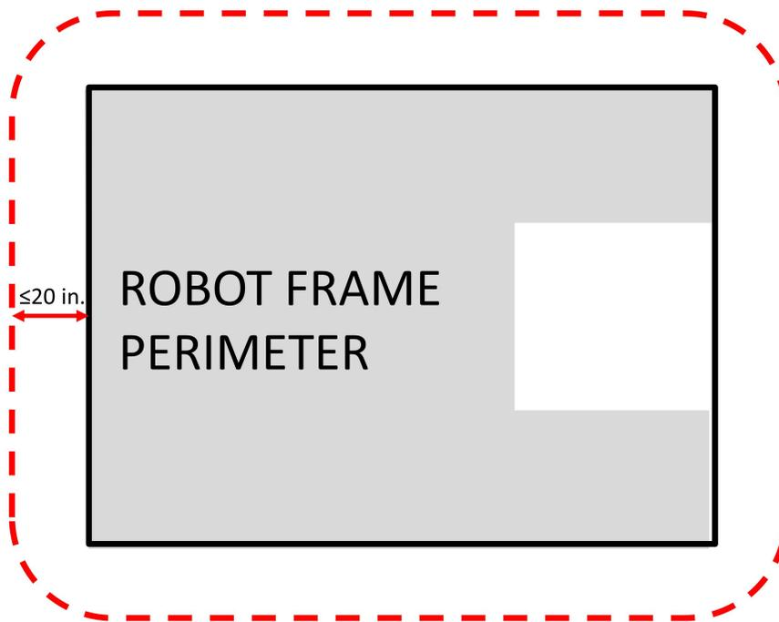
Figure 3-6: FRAME PERIMETER Extension
